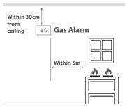
As Natural Gas is lighter than air it will naturally rise and build up at a high level in the room. The NG-9B alarm should therefore be placed above the highest window, door or vent in the room. Ideally within 30cm of the ceiling.
